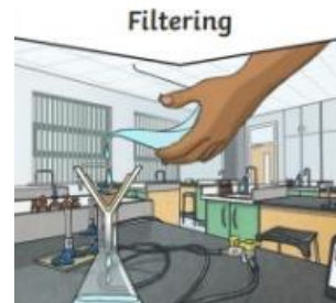
Solid particles get caught in the filter, liquid passes through.
